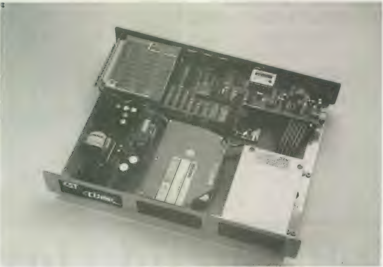
Inside: A steel chassis with optional single or dual disc drives, or Winchester drive combination.
